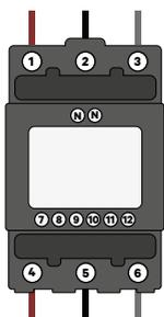
1. Now, wire the power meter. Connect the 3 phases (position 1-2-3 for power in, 4-5-6 for power out).
