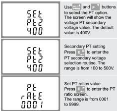
For example, if set the ratio to be 100, it means the primary voltage equals secondary voltage x100.
