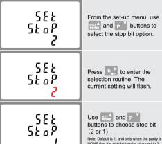
On completion of the entry procedure, press the setting and press  $\frac{1}{1000}$  to return to the main set up menu.
