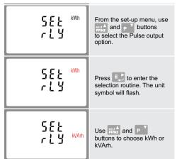
On completion of the entry procedure, press **E** to confirm the setting and press **W** to return to the main set up menu.
