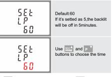
Press E to confirm the setting and press KA to return to the main set up menu.
